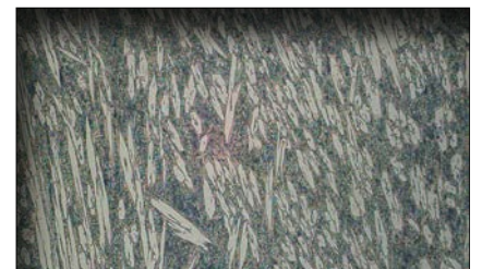
Inter-plate IP1200 AS/NZS 2576:2005 Austenitic Complex Chromium Carbide Overlay x 100 magnification
