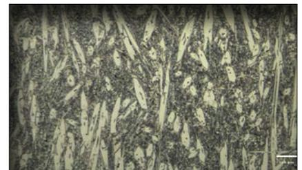
**Inter-plate IP800 AS/NZS 2576:1996 Austenitic Complex Chromium Carbide Overlay x 100 magnification**
